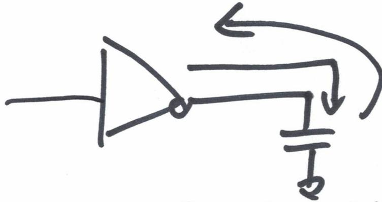
$$I_{avg} = \frac{Q_{tot}}{T} = \frac{V_{DD} C_{tot}}{T}$$
