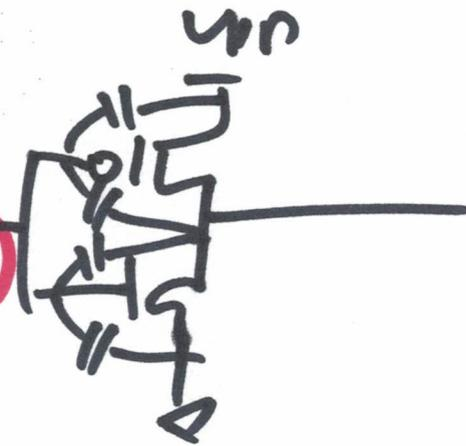
$$C_{in} = C_{inpt} + C_{inn} = \frac{3}{2} (C_{oxn} + C_{oxp})$$
