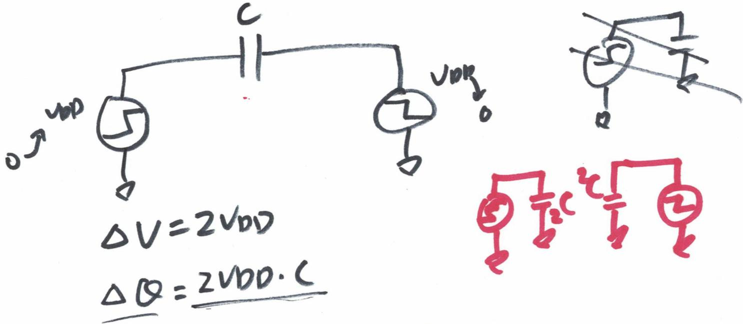
$$C_{eff} = \frac{\Delta Q}{v_{DD}} = \frac{2v_{DD} \cdot C}{v_{DD}} = 2C$$
