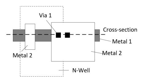
4. The following figure shows the top-view of a layout. Draw the cross-sectional views (cross-section 1 and cross-section 2 of the locations indicated by the dashed lines. (10 points)
