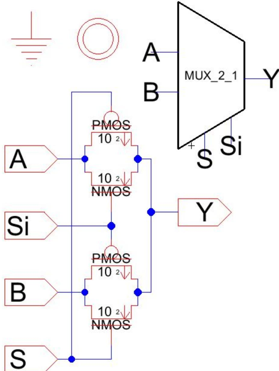
Checking schematic cell 'MUX\_2\_1{sch}'
