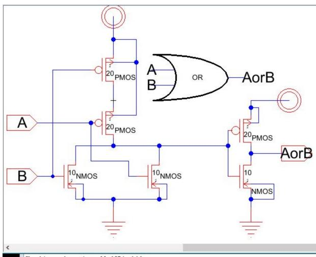
Checking schematic cell 'OR{sch}'
