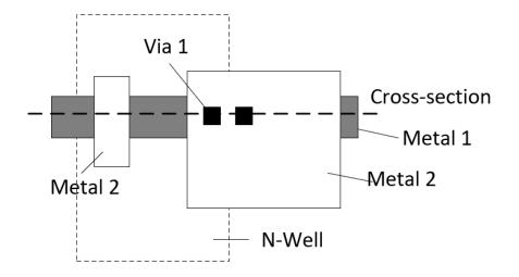
5. The following figure shows the top-view of a layout. Draw the cross-sectional views (cross-section 1 and cross-section 2 of the locations indicated by the dashed lines. (10 points)
